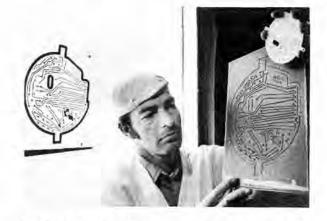
STAGES in the photochemical production of a printed circuit board are displayed by Jac Constant (4221-1). At left is a film negative of the master drawing, in the center is a template made from photopolymer, and in the upper right is a printed circuit board ready for installation of components. The new technique using photopolymers and chemical etching is described in the accompanying article.
